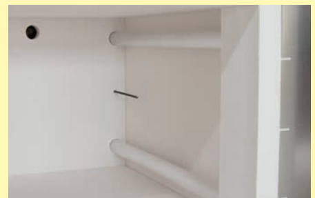
Heating elements protected in quartz glass tubes
